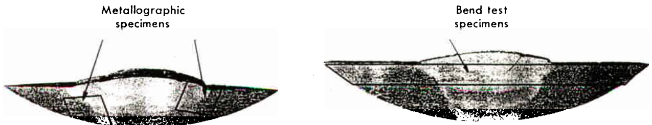
Fig. 2 Sections for metallographic examination and bend testing cut from boat-shaped slice
