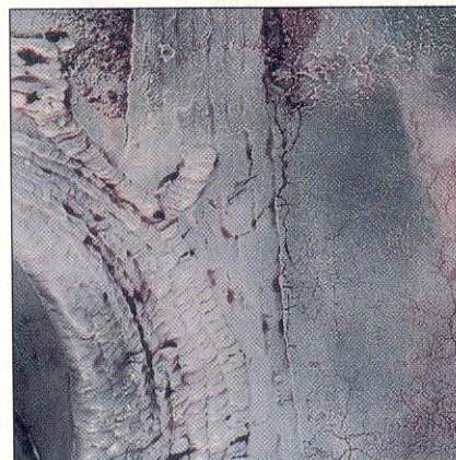
Upper left: Corrosion grooving apparent beneath pressure tap. Upper right: Stainless steel strip lining applied over integral stainless steel cladding.
