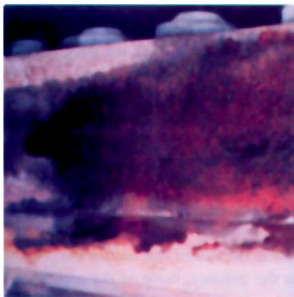
Fig. 1 (above): Corrosion product build up at the head to shell surface.
